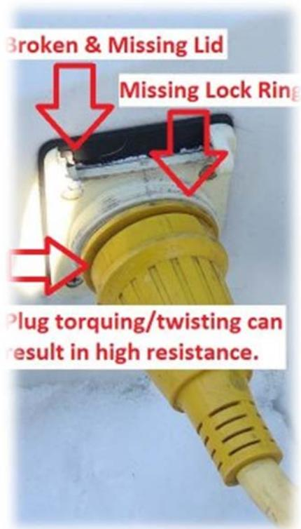
A likely place an electrical fire can start is at the boat's inlet receptacle. The inlet receptacle is the fixture on the side of the boat, with the hinged cap, where you connect the shore power cable. Since it is often exposed to the elements, the inlet receptacle's condition can deteriorate.
