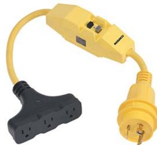
Be very careful when using extension cords with this equipment as they may become overheated if less than 10 AWG. Most power cords you buy even for outdoor use are 16 AWG. Heavy duty may be 12 AWG, but these will not be protected from overheating by the pedestal breaker. Check cable and connections regularly, they should not become excessively warm during use.
